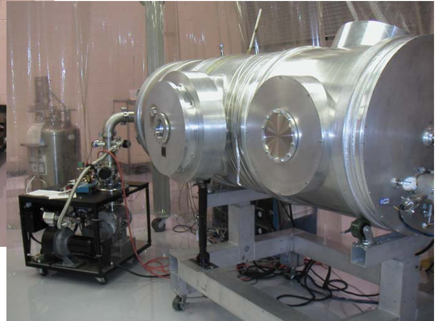
“MIC2” Multi-function IR Calibrator
